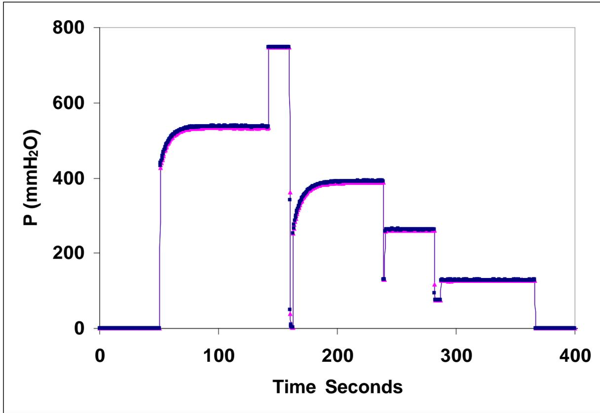
Figure 9. Simultaneous response of both transducers to a series of HRS tests.
