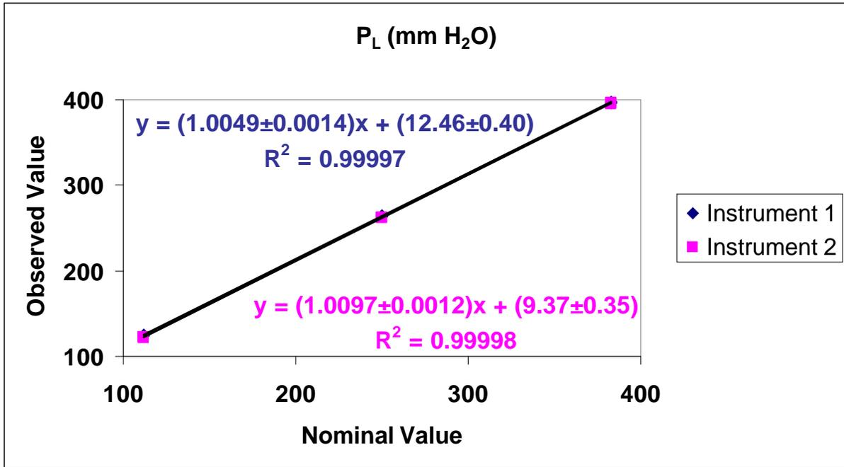
Figure 13. Comparison of  $P_L$  values from HRS tests with the nominal values after re-calibration of flow meters ( $n=5$ ).
