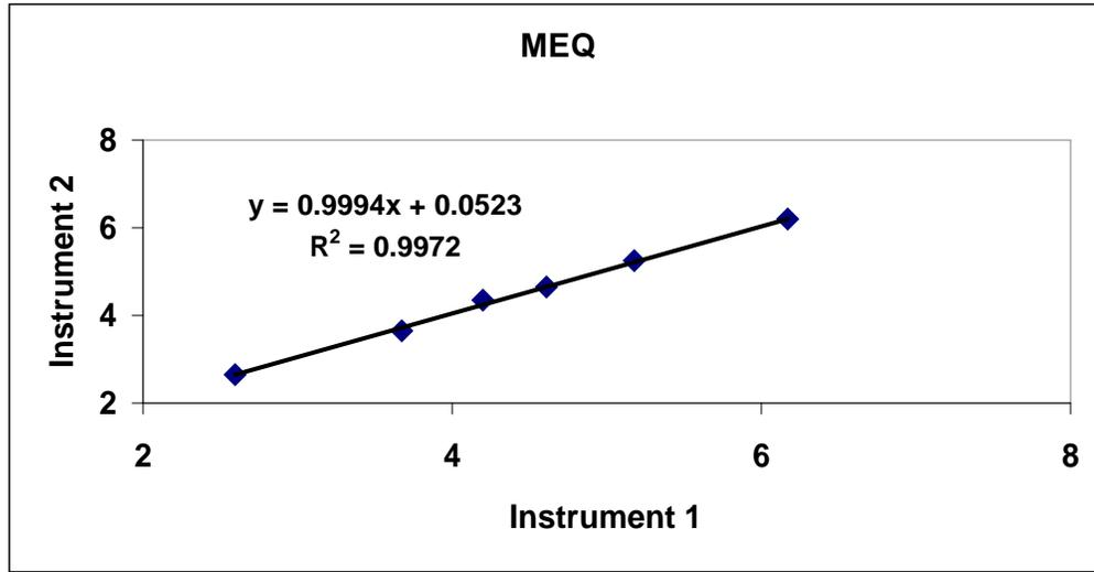
Figure 8. Average FMT Micronaire values comparing the performance of the two instruments for 6 different cottons (n= 5).
