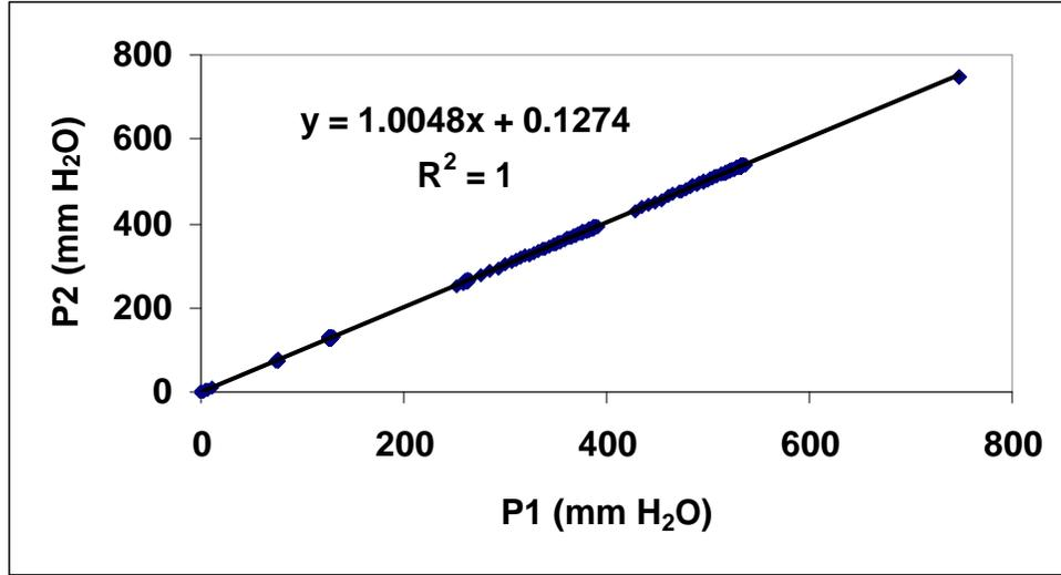
Figure 10. Comparison of the two pressure transducers using the data from Figure 9.
