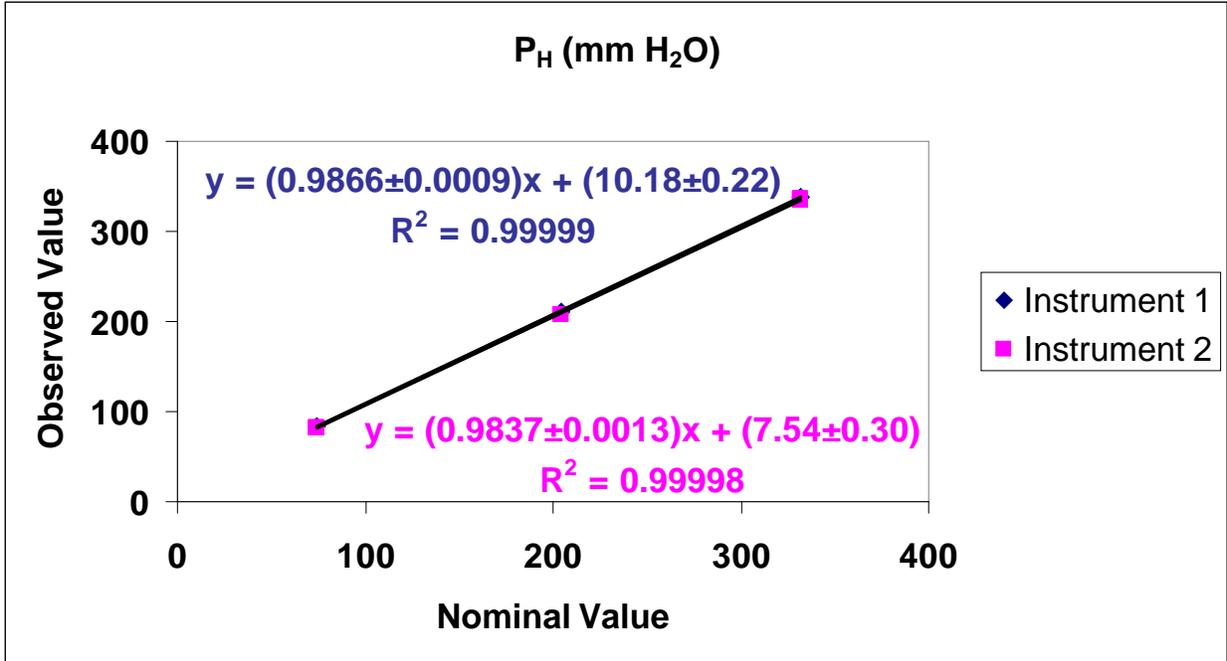
Figure 14. Comparison of P<sub>H</sub> values from HRS tests with the nominal values after re-calibration of flow meters (n=5).
