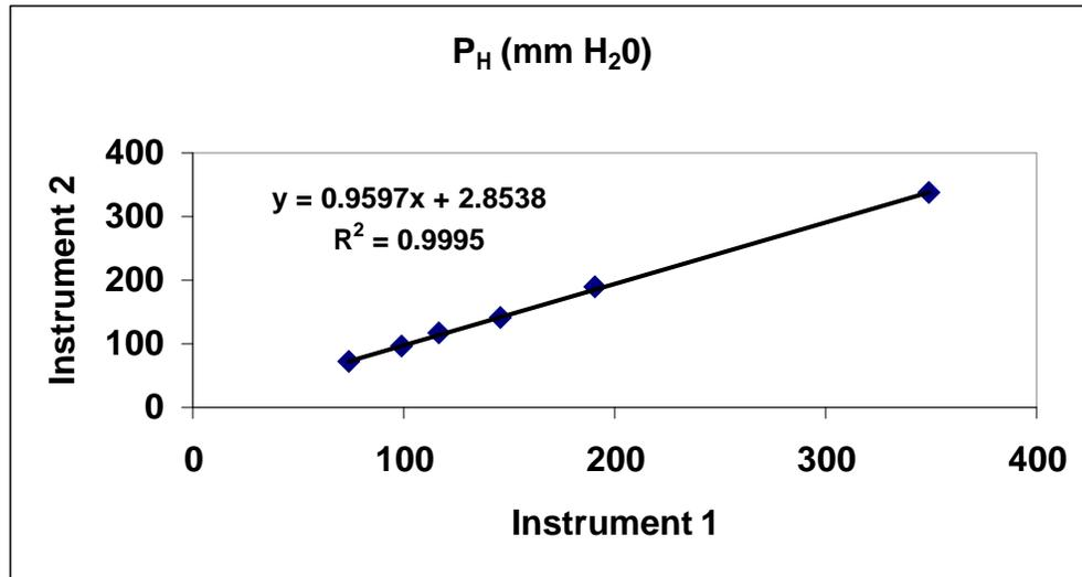
Figure 5. Average P<sub>H</sub> results comparing the performance of the two instruments for 6 different cottons (n = 5).
