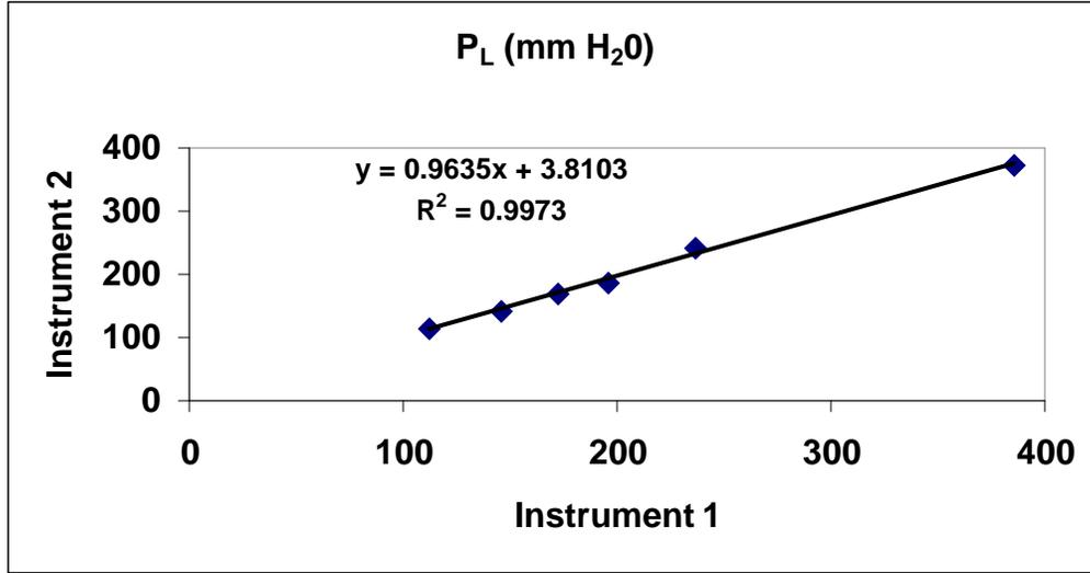
Figure 4. Average P<sub>L</sub> results comparing the performance of the two instruments for 6 different cottons (n = 5).
