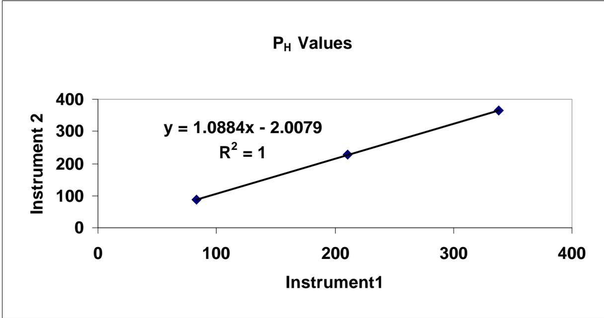
Figure 12. Comparison of the average  $P_H$  values ( $n=5$ ) from HRS tests with the initial (factory) calibration of flow meters.
