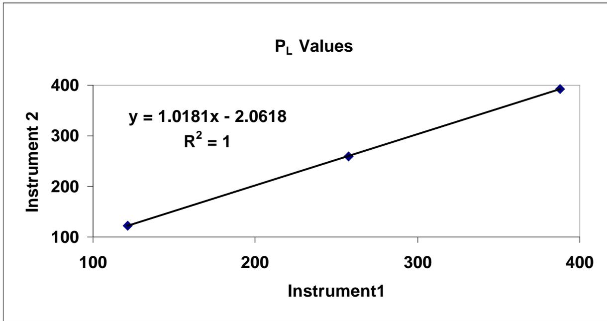
Figure 11. Comparison of average (n=5) P<sub>L</sub> values from HRS tests with the initial (factory) calibration of flow meters.
