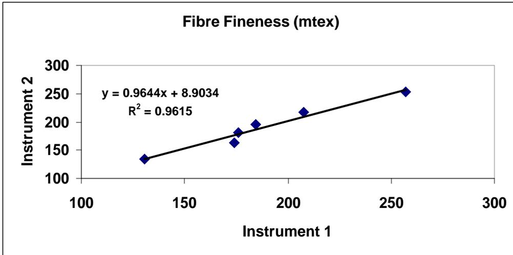
Figure 7. Average fiber fineness results comparing the performance of the two instruments for 6 different cottons (n=5).
