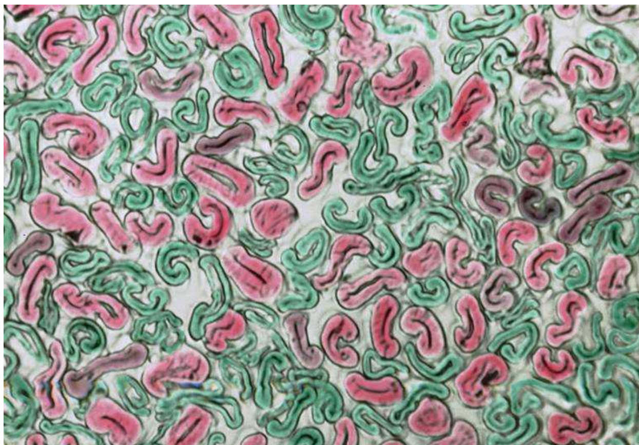
Figure 2. Cross sections (light micrograph) of cotton fibers dyed to show mature and immature fibers
