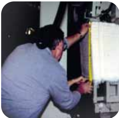
A study aimed at improving bale handling focused on bale size and density. This platen separation measurement taken at a New Mexico gin was part of the Beltwide data collection.
