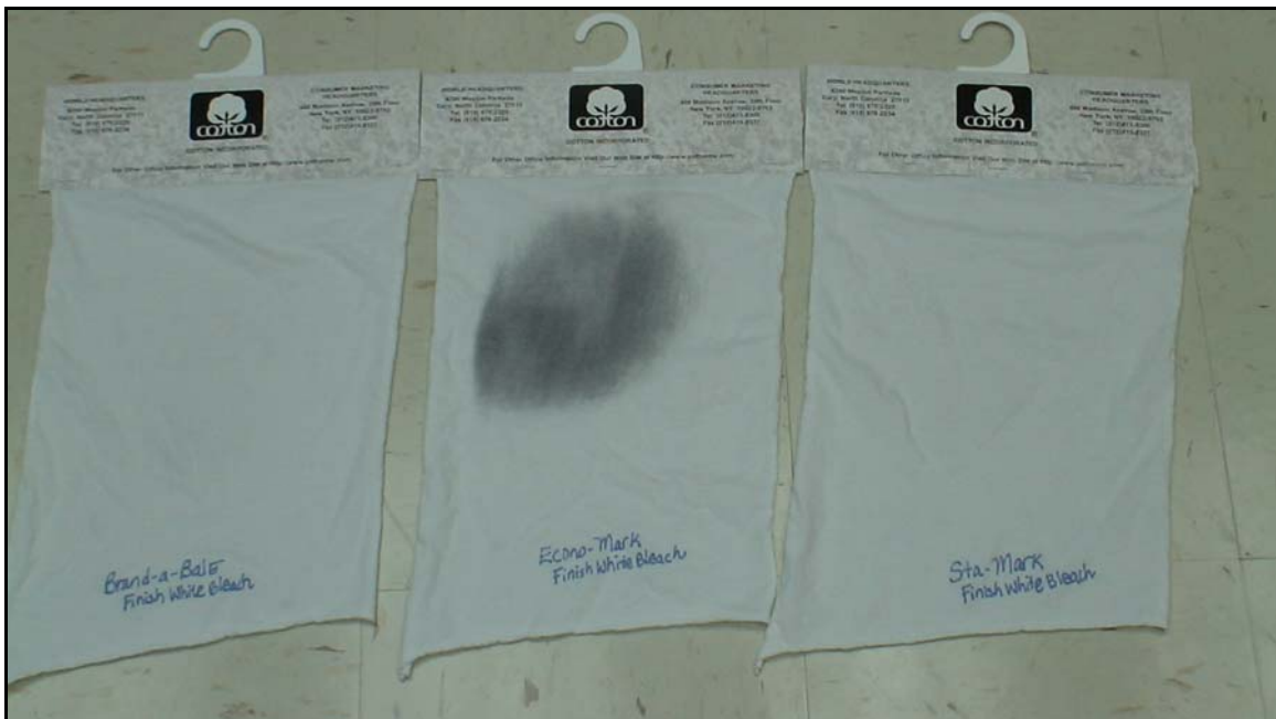
Figure 5: Sprayed fabric after finish white bleach (Left to Right: Brand-a-Bale, Econo-Mark, Sta-Mark)
