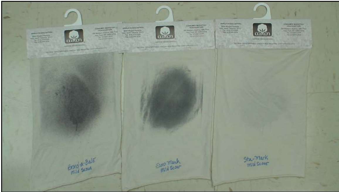
Figure 2: Sprayed fabric after mild scour using soda ash (Left to Right: Brand-a-Bale, Econo-Mark, Sta-Mark)
