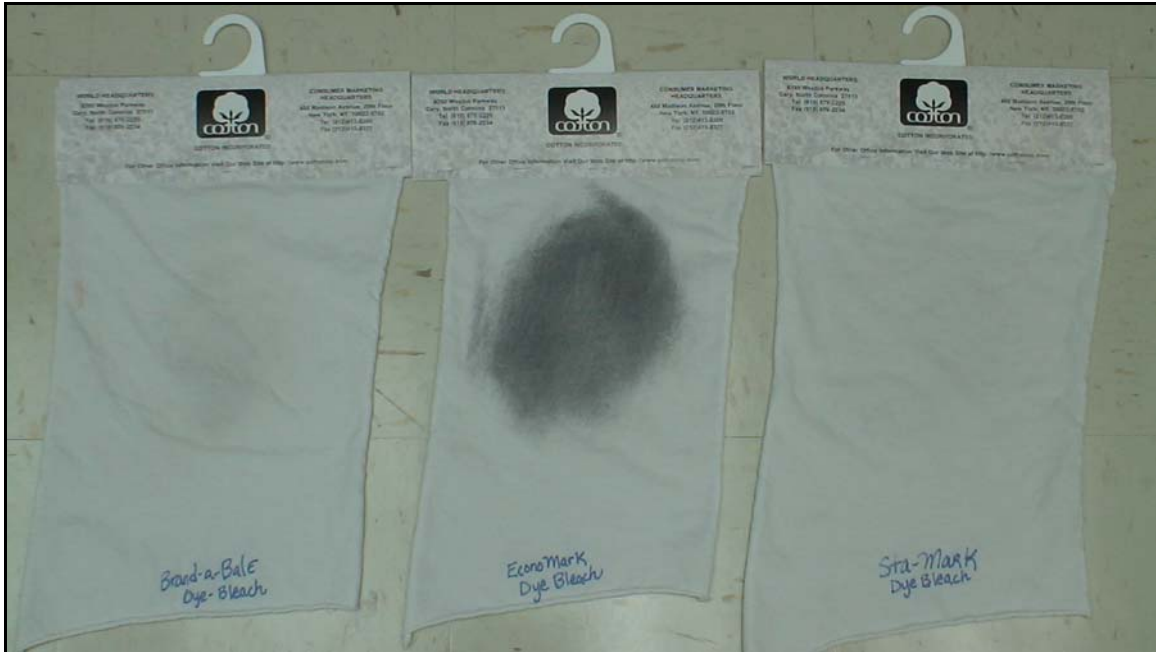
Figure 4: Sprayed fabric after dye based bleach (Left to Right: Brand-a-Bale, Econo-Mark, Sta-Mark)
