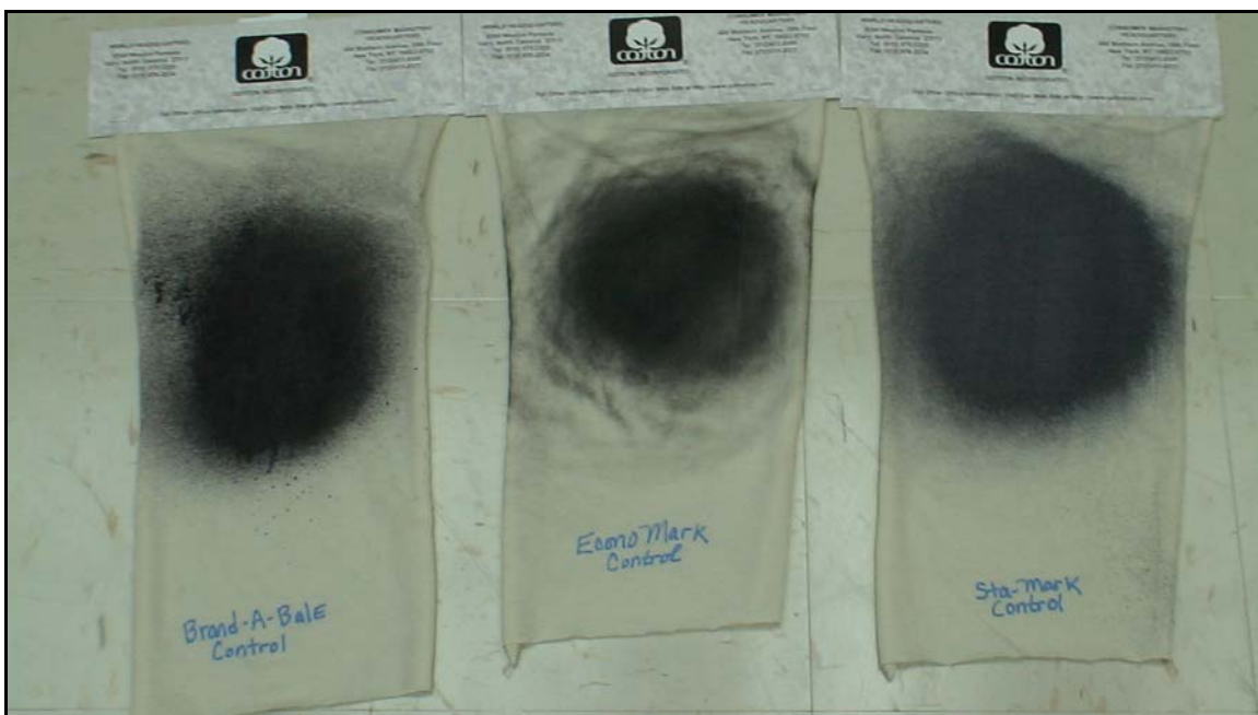
Figure 1: Sprayed fabric controls after drying (Left to Right: Brand-a-Bale, Econo-Mark, Sta-Mark)
