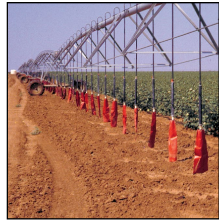
Figure 5. Center pivot sprinkler types. High pressure overhead nozzle (left) and low-pressure drop nozzle sprinkler (right).
