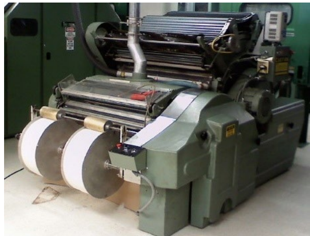
Figure 2. Front side of the carding machine showing collecting drums with carded web.
