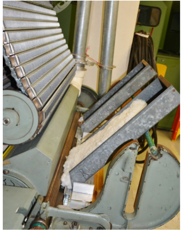
Figure 1. Back side of the carding machine with feed tray.
