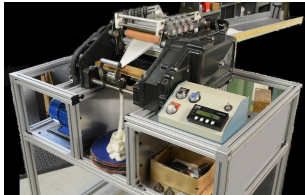
Figure 3. Modified draw frame with metal feed tray at the back and revolution counter at the front.
