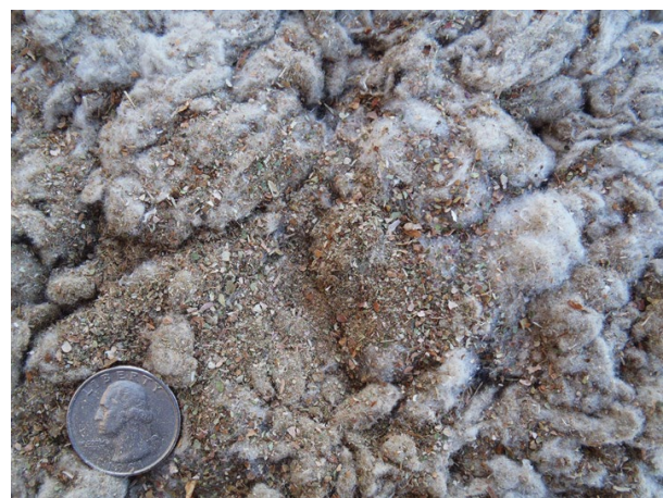
Figure 3. Photograph of typical trash captured by the mote cleaner system cyclones.
