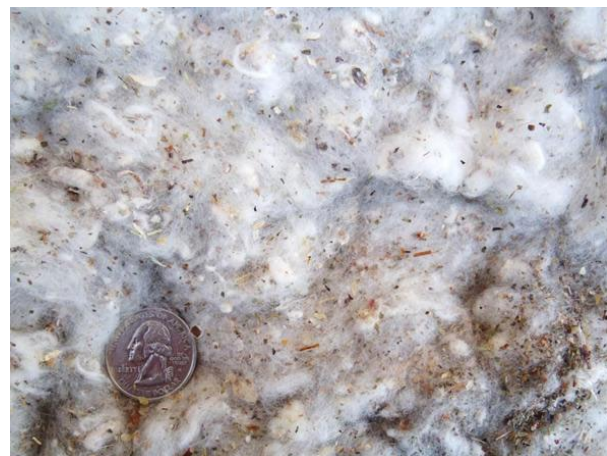
Figure 3. Photograph of typical trash captured by the 2 nd stage mote system cyclones.
