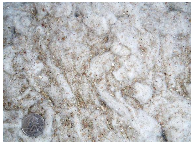
Figure 3. Photograph of typical trash captured by the cyclone robber system cyclones.
