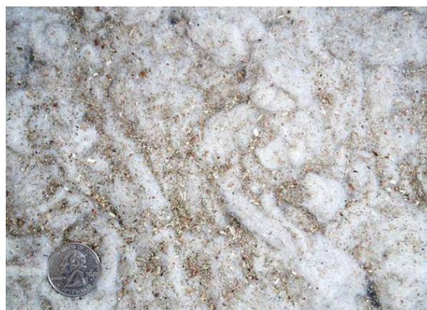
Figure 3. Photograph of typical trash captured by the 2 nd stage lint cleaning system cyclones.
