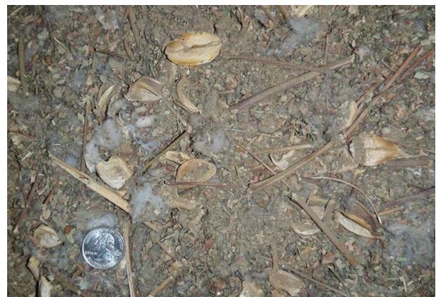
Figure 3. Photograph of typical trash captured by the 2 nd stage seed-cotton cleaning system cyclones.
