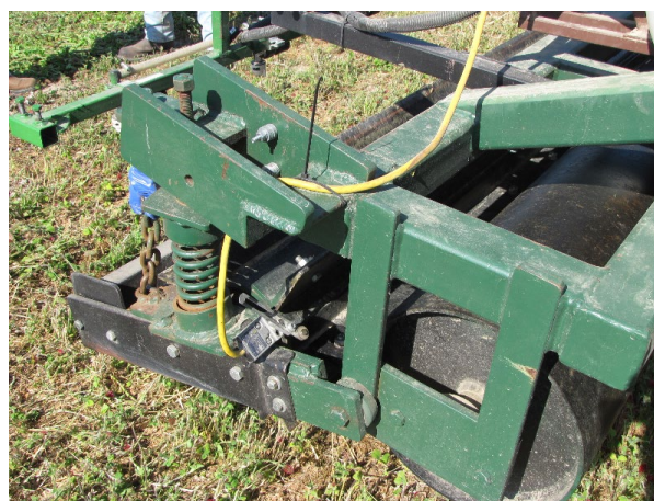
Figure 3. Two-stage roller/crimper with electric switch mounted on the pivoted roller's frame to be energized by the 12.7 mm (½ inch) diameter engagement bars mounted on the crimping bars of the crimping drum.
