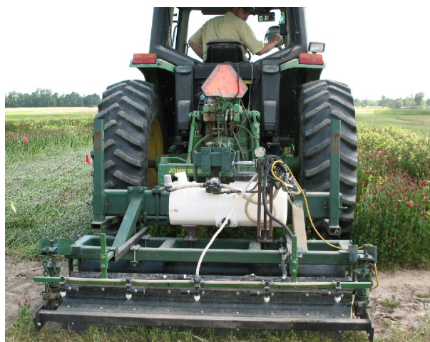
Figure 1. Two-stage roller/crimper (Kornecki, 2011, U.S. Patent Number 7,987,917 B1) with 53 L plastic tank and boom with five nozzles each controlled by fast acting solenoid valve to discharge herbicides on crimped cover crop residue.
