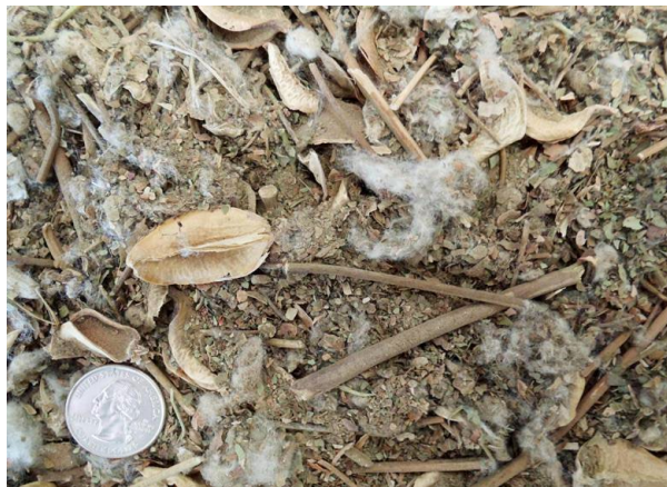
Figure 4. Photograph of typical trash captured by the 1 st stage seed-cotton cleaning cyclones.
