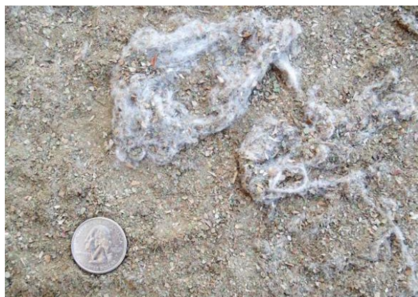
Figure 4. Photograph of typical trash captured by the unloading system cyclones.
