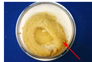
Figure 14. EPA Method 17 filter from the overflow system with lint fibers (indicated by arrow).
