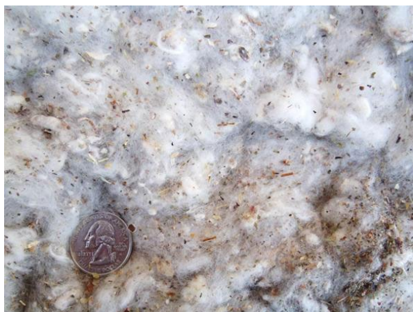
Figure 4. Photograph of typical trash captured by the combined mote system cyclones.
