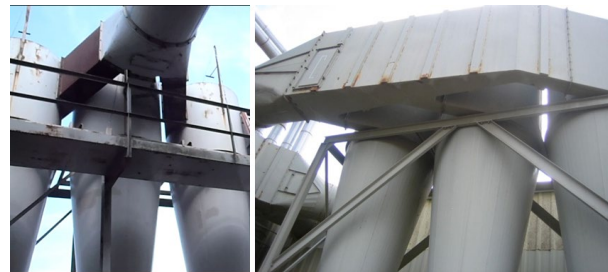
Figure 12. Photographs triple cyclone configurations (left to right): triple cyclone configuration with flow split among three, side-by-side, identical cyclones; triple cyclones in a tandem configuration with flow split among three, one-behind-another, identical cyclones.
