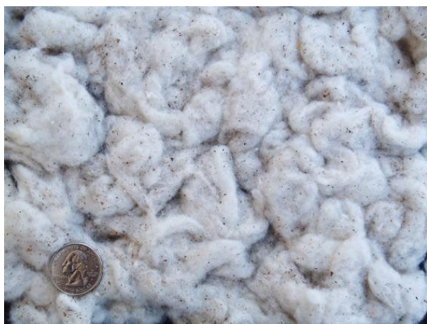
Figure 4. Photograph of typical trash captured by the battery condenser system cyclones.
