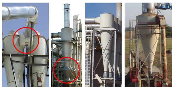
Figure 10. Cyclone design variations for the tested systems (left to right): dual configuration that splits flow between identical 1D3D cyclones with 2D2D inlets; 1D3D cyclone with 2D2D inlet and expansion chamber on the cone; 1D3D cyclone with 2D2D inlet and standard cone; ½D2D cyclone with a square inlet measuring about ¼D on a side.
