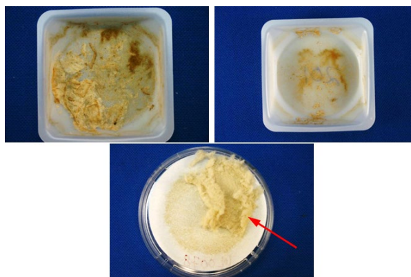
Figure 14. EPA Method 201A filter and sampler head acetone washes from the 1 st stage lint cleaning system with lint fiber on the filter (indicated by arrow). Clockwise from top left: > 10 µm wash, ≤ 10 µm wash, and filter.
