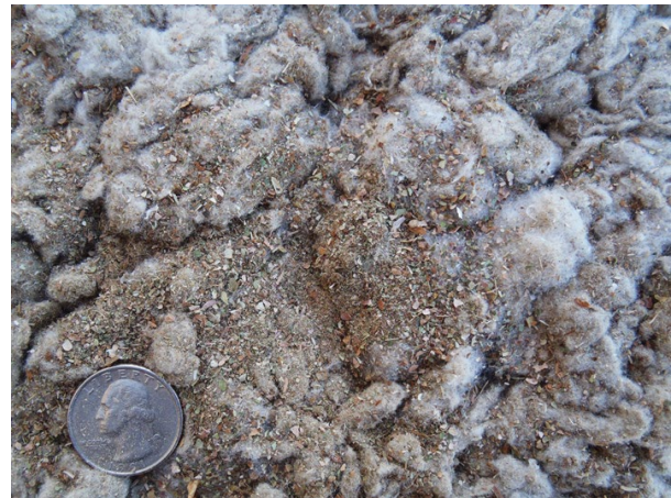
Figure 4. Photograph of typical trash captured by the overflow system cyclones.
