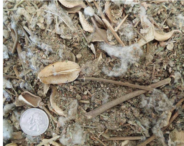
Figure 4. Photograph of typical trash captured by the master trash system cyclones.
