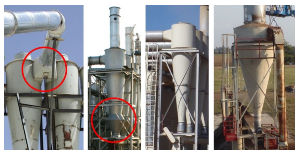
Figure 10. Cyclone design variations for the tested systems (left to right): dual configuration that splits flow between identical 1D3D cyclones with 2D2D inlets; 1D3D cyclone with 2D2D inlet and expansion chamber on the cone; 1D3D cyclone with 2D2D inlet and standard cone; \frac{1}{2} D2D cyclone with a square inlet measuring about \frac{1}{4} D on a side.
