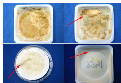
Figure 12. Atypical EPA Method 201A filter and sampler head acetone washes from the master trash system with lint fiber in the 10 to 2.5 μm and 2.5 μm washes and on the filter. Clockwise from top left: > 10 μm wash, 10 to 2.5 μm wash, ≤ 2.5 μm wash, and filter.
