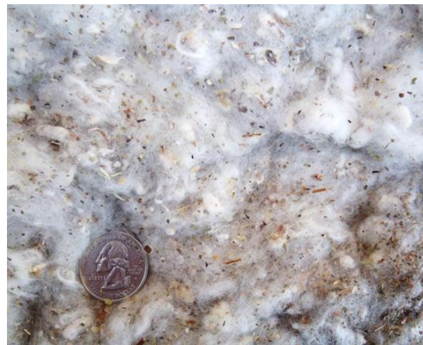
Figure 4. Photograph of typical trash captured by the mote cyclone robber cyclones.
