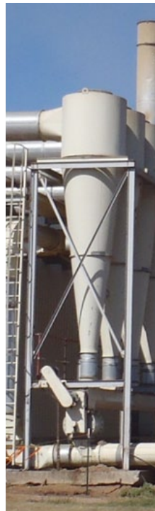
Figure 12. Cyclone design for the tested systems: 1D3D cyclone with 2D2D inlet and standard cone.
