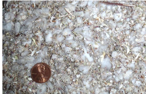
Figure 4. Photograph of typical trash captured by the mote cleaner system cyclones.
