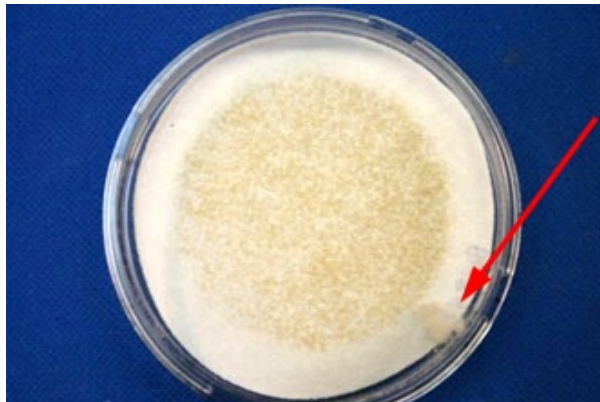
Figure 13. Atypical EPA Method 201A filter from the combined mote system with lint.
