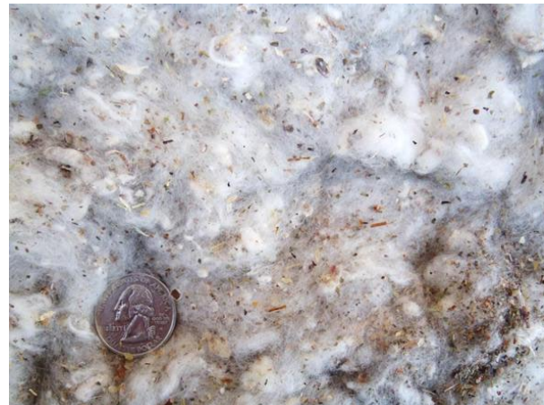
Figure 4. Photograph of typical trash captured by the 2 nd stage mote system cyclones.
