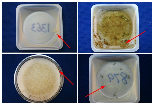
Figure 16. Atypical EPA Method 201A filter and sampler head acetone washes from the 2 nd stage mote system with lint in all three washes and on the filter. Clockwise from top left: > 10 \mu\text{m} wash, 10 to 2.5 \mu\text{m} wash, \leq 2.5 \mu\text{m} wash, and filter.
