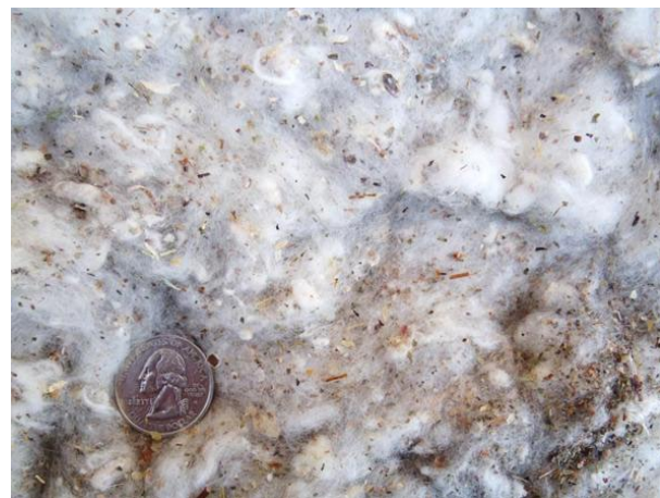
Figure 4. Photograph of typical trash captured by the first-stage mote system cyclones.
