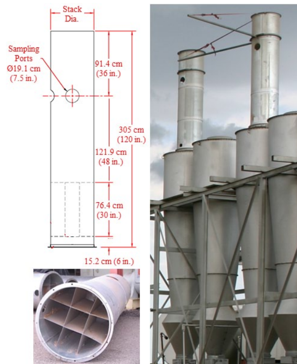
Figure 8. Schematic and photographs of stack extensions with sampling port and straightening vanes (rail attached to extension above sampling port, at right, supports sampling probe during testing traverse).
