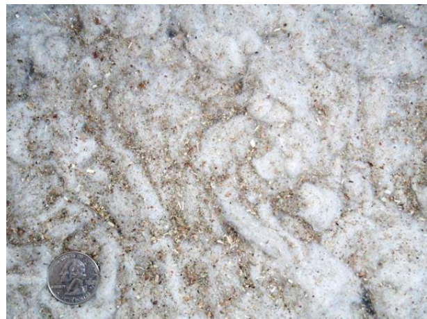
Figure 4. Photograph of typical trash captured by the cyclone robber system cyclones.
