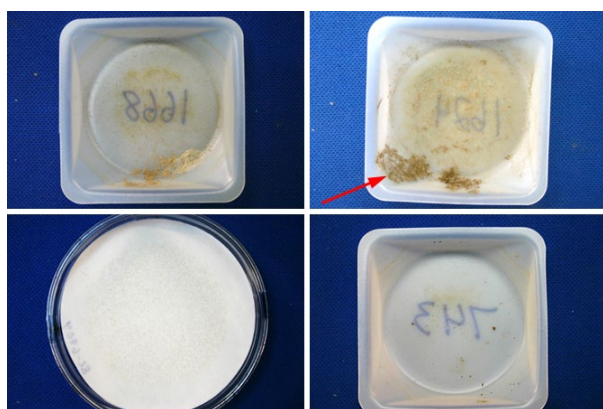
Figure 14. Atypical EPA Method 201A filter and sampler head acetone washes from the combined lint cleaning system; lightly loaded with lint fiber in the 10 to 2.5 \mu\text{m} wash. Clockwise from top left: > 10 \mu\text{m} wash, 10 to 2.5 \mu\text{m} wash, \leq 2.5 \mu\text{m} wash, and filter.
