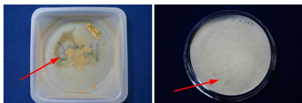
Figure 14. Atypical EPA Method 201A filter and sampler head acetone wash from the 2 nd stage lint cleaning system with lint fiber in the 10 to 2.5 \mu\text{m} wash and on the filter. Left to right: 10 to 2.5 \mu\text{m} wash and filter.
