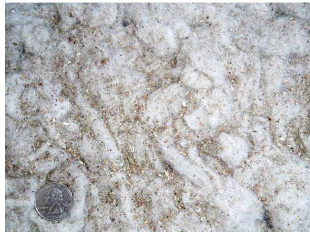
Figure 4. Photograph of typical trash captured by the 1 st stage lint cleaning system cyclones.
