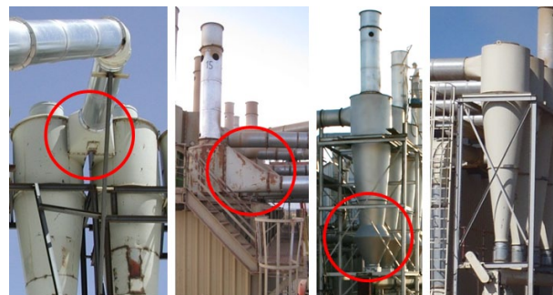
Figure 15. Cyclone design variations for the tested systems (left to right): dual configuration that splits flow between identical 1D3D cyclones with 2D2D inlets; 1D3D cyclone with an inverted 1D3D inlet; 1D3D cyclone with 2D2D inlet and expansion chamber on the cone; 1D3D cyclone with 2D2D inlet and standard cone.
