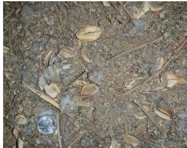
Figure 4. Photograph of typical trash captured by the 2 nd stage seed-cotton cleaning system cyclones.
