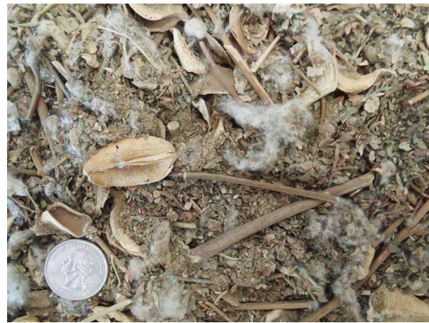
Figure 4. Photograph of typical trash captured by the 1 st stage seed-cotton cleaning system cyclones.
