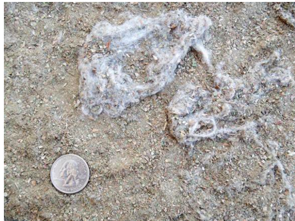
Figure 4. Photograph of typical trash captured by the unloading system cyclones.
