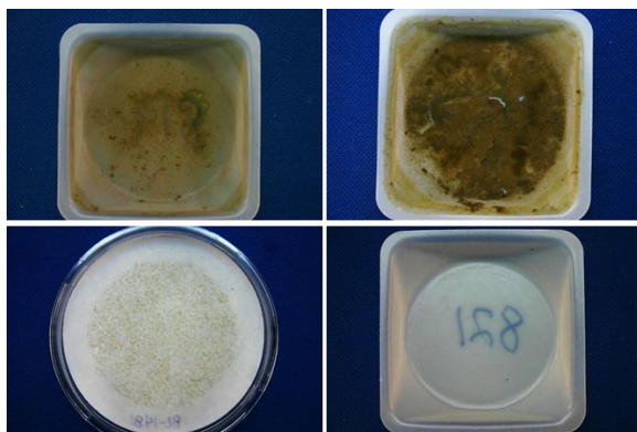
Figure 13. Typical EPA Method 201A filter and sampler head acetone washes from the unloading system. Clockwise from top left: > 10 μm wash, 10 to 2.5 μm wash, ≤ 2.5 μm wash, and filter.
