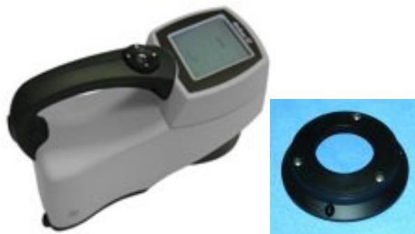
Figure 2. HunterLab MiniScan EZ (MSEZ) portable spectrophotometer and glass-covered 30-mm sampling port.
