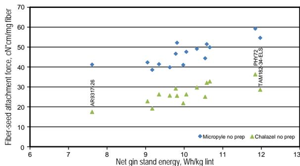
**Figure 4. Net gin stand energy for 15 genotypes vs. fiber-seed attachment force measured for micropyle and chalazal tufts without prep.**
