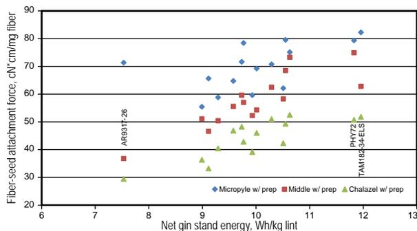
**Figure 5. Net gin stand energy for 15 genotypes vs. fiber-seed attachment force measured for micropyle, middle, and chalazal tufts with prep.**
