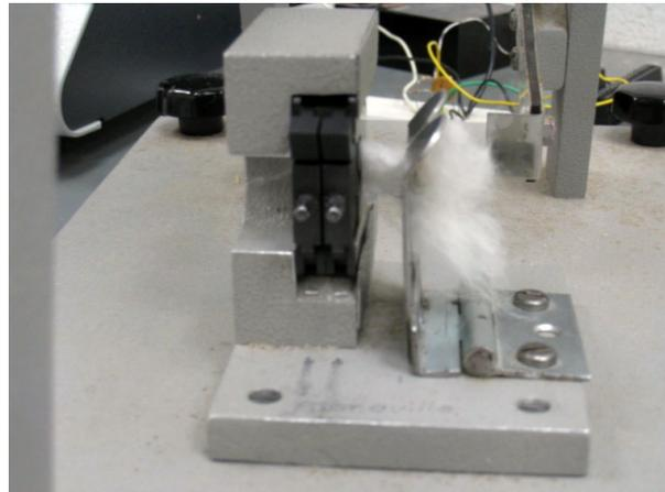
**Figure 2. Sample cartridge holding seed behind slotted seed plate (right side of pendulum path) and fiber bundle in clamps (left side of pendulum path).**
