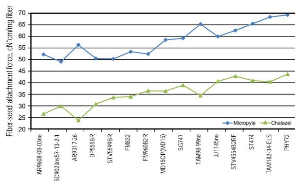
**Figure 3. Fiber-seed attachment force measured for 15 genotypes for micropyle tufts (averaged over prep) and chalazel tufts (averaged over prep).**
