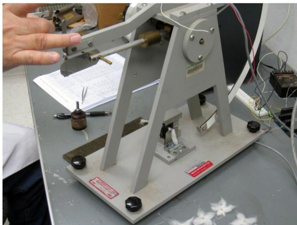
**Figure 1. Fiber-seed attachment force tester just before releasing the pendulum. Pendulum arm locked in raised position and sample cartridge in place. Note the prepared seed with four bundles (two chalazal and two micropyle) in the lower portion of the picture. Seed including middle tufts are not shown.**
