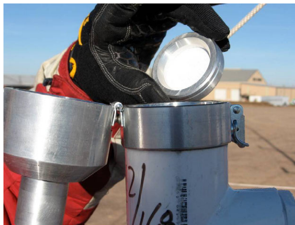
Figure 17. Filter cassette with clean filter being deployed in an ambient air sampler.
