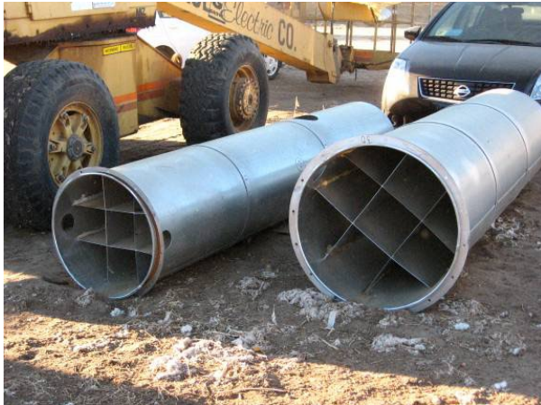
Figure 7. Stack extension with straightening vanes.
