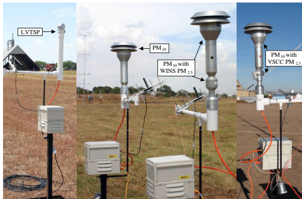
Figure 11. Low-volume (16.7 lpm target flow rate) stand-alone samplers equipped with a TAMU-USDA total suspended particulate (LVTSP) sampler head, a PM 10 sampler head, a Well Impactor Ninety-Six (WINS) PM 2.5 sampler head, and a very sharp cut cyclone (VSCC) PM 2.5 sampler head.
