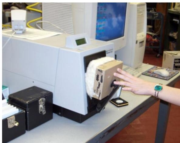
Figure 2. Example of color measurements with hand-applied pressure.
