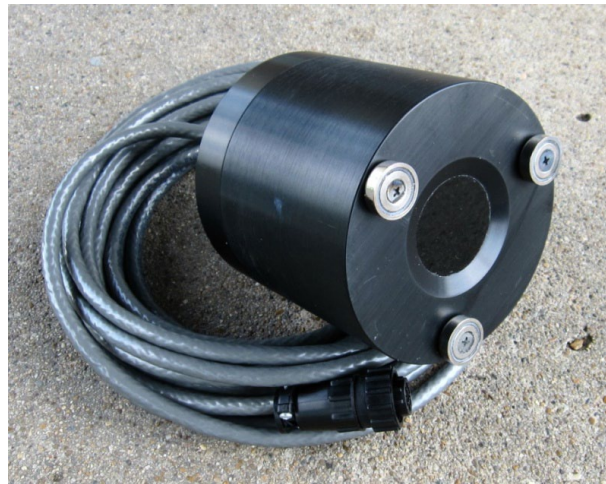
Figure 1. Mass flow sensor for gins.
