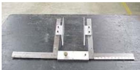
**Fig. 3.** Two carpenter squares joined together using a sliding mechanism with setscrews was used to measure hump thickness. Wide flanges were added to assist in measuring.
