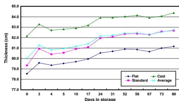
Fig. 5. Thickness of the bale averaged across all seven “humps” as a function of days in storage for the three types of platens for Phase I.
