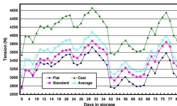
**Fig. 4.** Bale tie tension as a function of days in storage for the three types of platens in Phase I.
