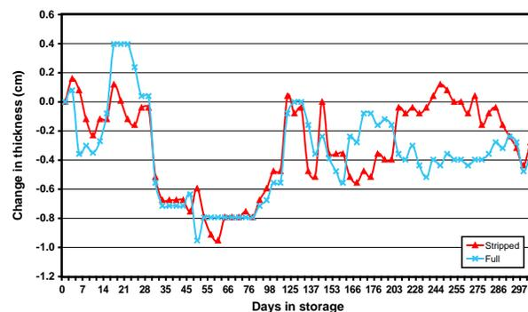
Fig. 11. Bale thickness (cm) at humps for the strip-coated and fully coated bales for days in storage at 21.1 °C (70 °F) and 50% RH for Phase III.
