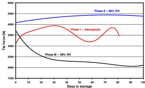
**Fig. 13.** Means for tie force (N) across Phase I, Phase II, and Phase III. Data for days 100-305 in Phase III were not substantially different from day 100 and are not shown in order to provide adequate resolution in this figure.
