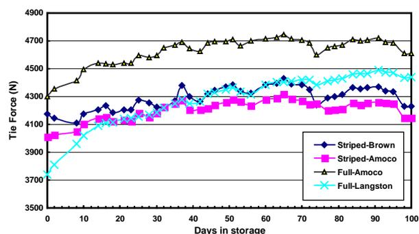
Fig. 7. Tie force (N) as a function of days in storage at 26.7 °C (80 °F) and 80% RH for universal density bales covered in four types of bagging for Phase II.
