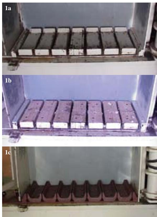
**Fig. 1.** Bottom platens used in pressing the bales. Shown are A.) Standard bottom platen for Continental Bespress. Note the outside edges of the platens are turned up to make it easier to insert the bale ties. B.) Standard platen with wooden inserts to create a flat platen. Similar inserts were used on the top platen for all treatments. C.) Cast steel platen.
