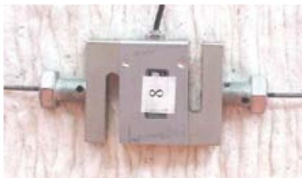
**Fig. 2.** Transducer installed in bale tie to measure bale tie forces.
