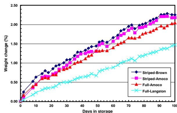
Fig. 6. Weight gain (%) as a function of days in storage at 26.7 °C (80 °F) and 80% RH for universal density bales covered in four types of bagging for Phase II.
