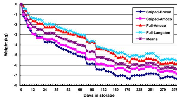
Fig. 9. Bale weight change (kg) as a function of days in storage at 21.1 °C (70 °F) and 50% RH for Phase III.
