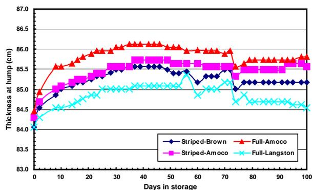
Fig. 8. Thickness at hump (cm) as a function of days in storage at 80 °C and 80% RH for universal density bales covered in four types of bagging for Phase II.
