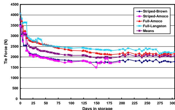
Fig. 10. Tie force (N) as a function of days in storage at 21 °C (70 °F) and 50% RH for Phase III.
