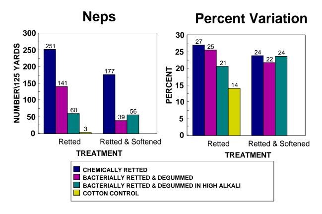
Figure 1. Yarn uniformity as measured with evenness tester from Zellweger Uster.
