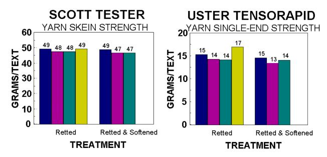
Figure 2. Yarn strength as measured with strength tester (Scott) and Tensorapid (Zellweger Uster).
