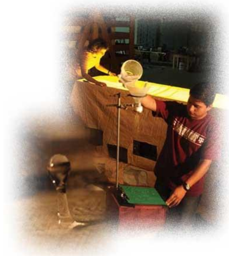
A rainfall simulation by Texas A&M University researchers determines moisture penetration of a module cover sample.
