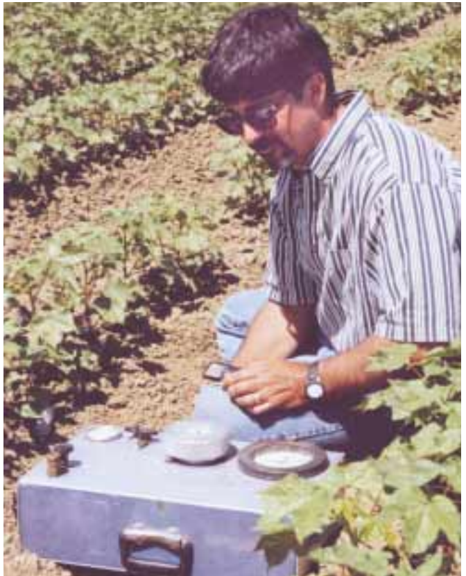
To help in irrigation decision-making, crop consultant Jim Hill uses a pressure bomb to measure leaf water potential of plants on Ted Sheely's California farm as part of a hyperspectral remote sensing research project.
