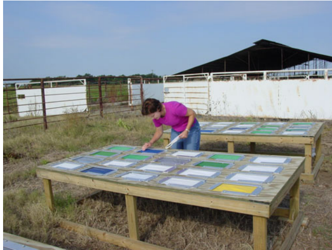
Figure 3. Specimen in outdoor weathering racks.
