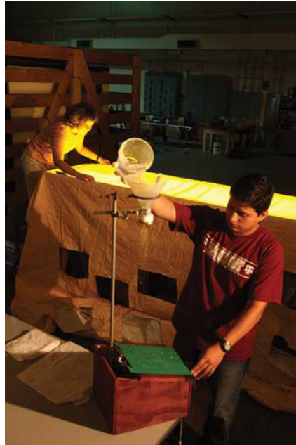
Figure 1. Rainfall simulation in the foreground and light table evaluation in the background.
