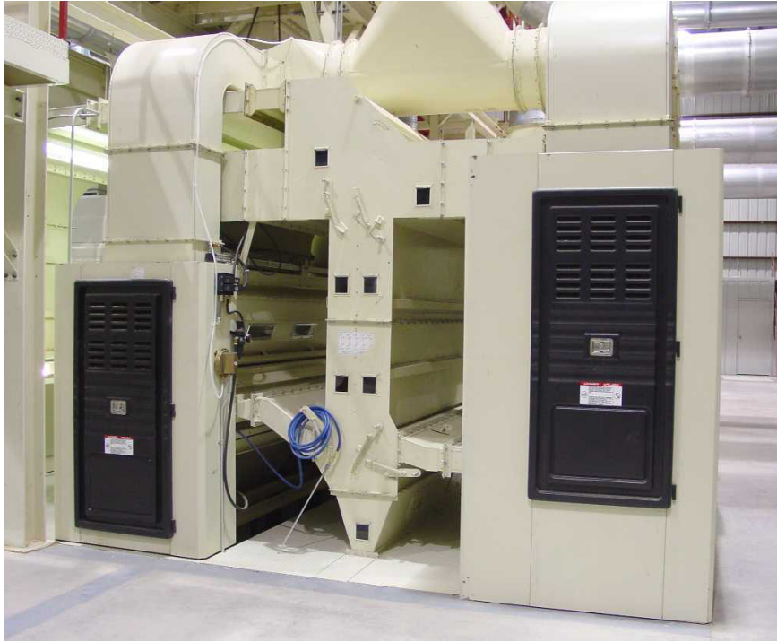
Figure 2. Sentinel™ Lint cleaner (left) and Model 108 Lint cleaner (right) installation at North Gin Ltd.
