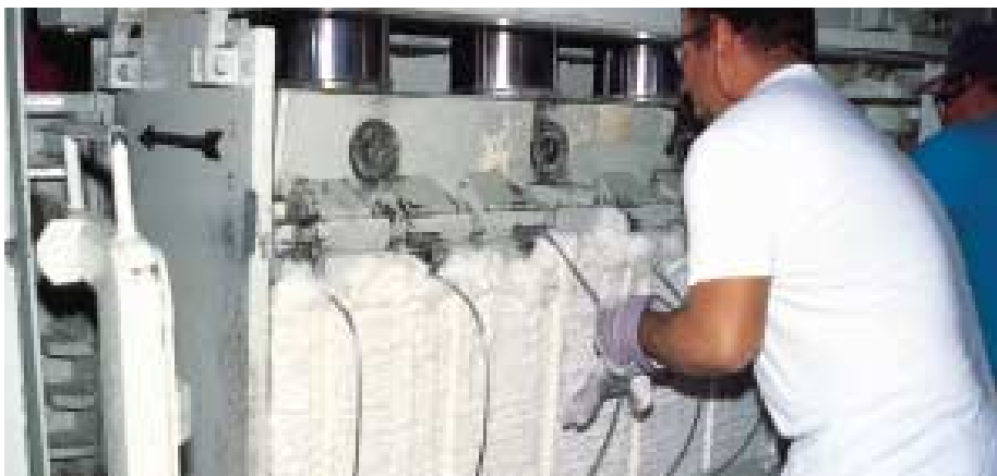
The Joint Cotton Industry Bale Packaging Committee monitored recessed tie test programs with a goal of decreasing the potential of lint contamination.
